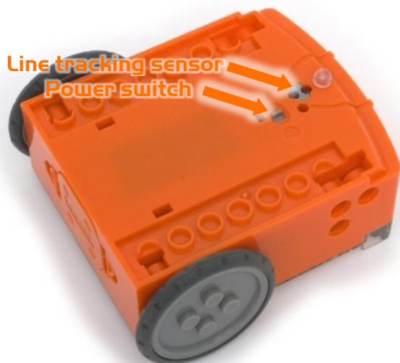
Edison's power switch and line tracking sensor
