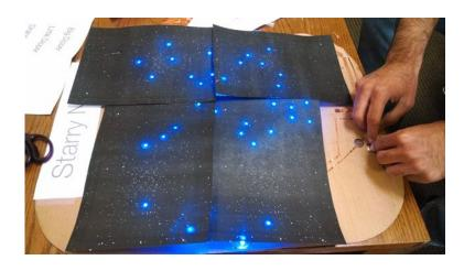
It is important to first sketch out the entire sky (circuit) - where all the stars (Blue LEDs) go, where each of the constellation (Blue LEDs with Green edges) goes. Once you have figured that out, draw this circuit on a piece of cardboard. All the Blue LEDs will be connected in parallel on the main circuit
